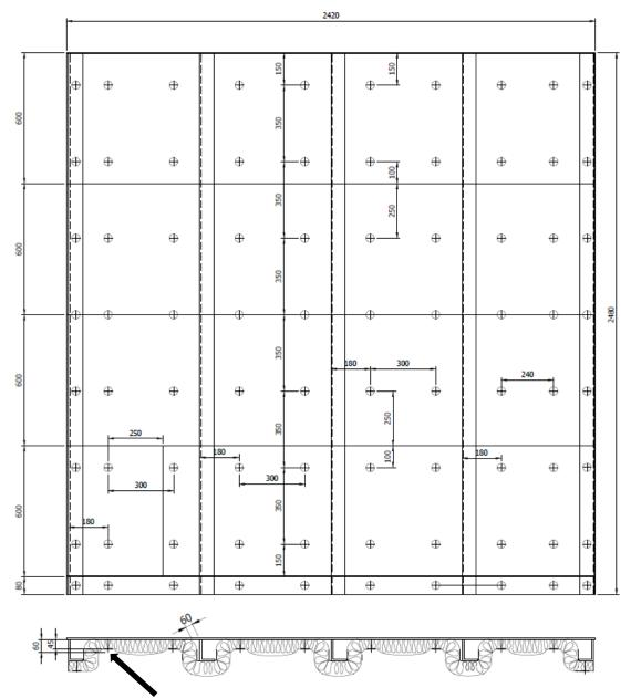
Blanket may be compressed from 65mm up to 45mm (i.e. 30%) thickness. Pin length to be from 50mm to 80mm typically.
