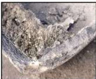
Fig. 5 – Dross accumulation in this crucible caused the crucible to fail because of expansion cracking
