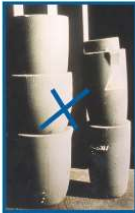
Fig. 1 – Stacking crucibles, one inside the other, will damage the crucibles.
