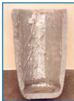
Fig. 3a – Metal with a high flux concentration caused Corrosion of lower internal wall of this crucible
