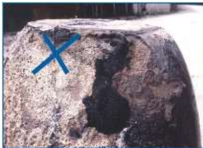
Fig. 4 – Direct contact with a burner flame caused this oxidation damage. The base block holding the crucible was not the proper height
