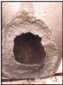
Fig. 3 – Cone shaped fracture caused by the impact of charge materials dropped into the inside of the crucible.
