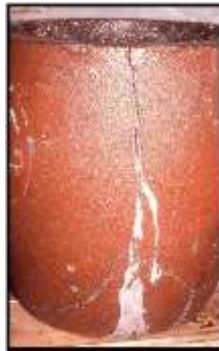
Fig. 2 – Typical Y shaped crack. This crucible cracked because the charge materials were packed so tightly that there was no space for their expansion when heated
