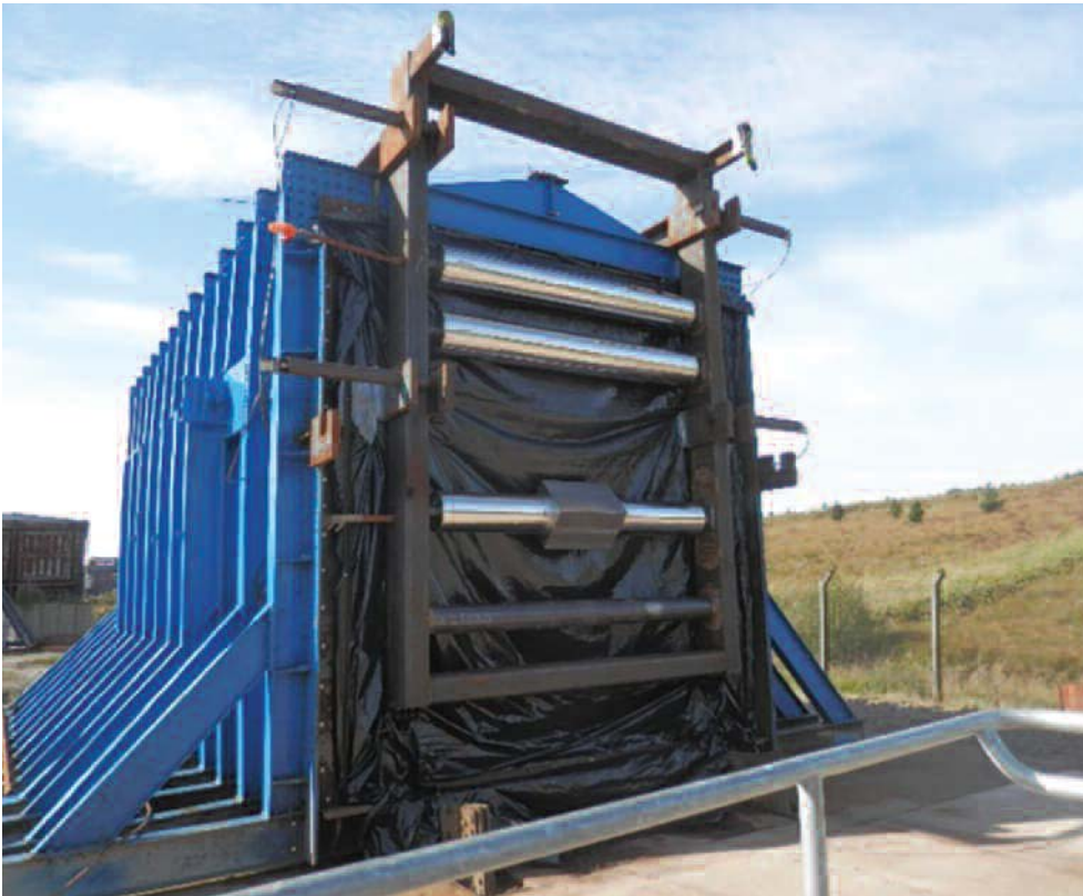
Pipes and RES system installed in explosion chamber prior to explosion testing.
