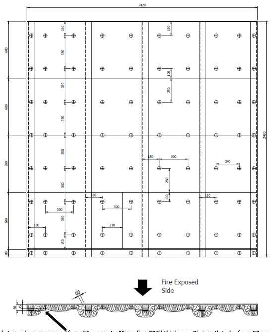
Blanket may be compressed from 65mm up to 45mm (i.e. 30%) thickness. Pin length to be from 50mm to 80mm typically. Blanket may be compressed to 25mm over the stiffener flange.
