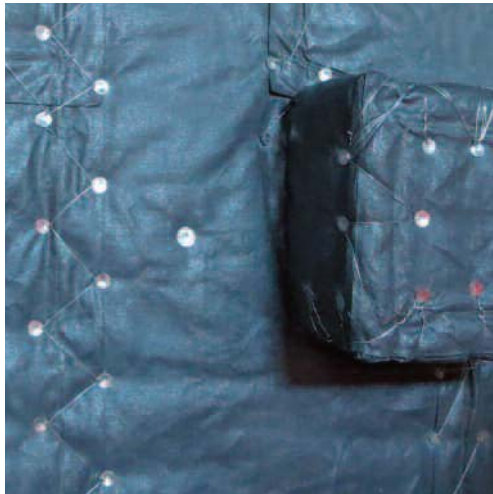
Raised corner detail used in jet fire test specimen
